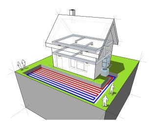
**Ground-source heat pumps** use underground pipes, known as ground loops, to extract heat from the earth. These loops are filled with a heat-transfer fluid that absorbs heat from the ground and carries it to the heat pump. Ground-source heat pumps offer high efficiency and consistent performance since the ground temperature remains relatively stable throughout the year. However, they require more upfront investment because ground loops must be installed.
